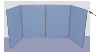
Take the 1st set of 4 panels (with connecting clips) and open out until the above shape is achieved (Ensure the connecting clips are at the top of the panels)
